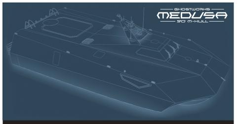
Medusa, built on our 27 Meter M-Hull platform, combines advanced naval architecture with carbon fiber construction for unmatched speed, stability, and payload flexibility in harsh environments. Her waterjet propulsion, subsystem-agnostic design, and multipurpose launch bay enable rapid reconfiguration for ISR, special ops, mine clearance, SAR, or unmanned systems—supporting up to 15 crew for single-day or extended multi-role operations.
